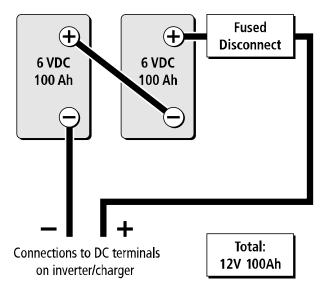
Figure 12 Batteries Connected in Series
